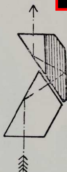
Dialyt Roof Prism System of the DIALYT Binoculars
