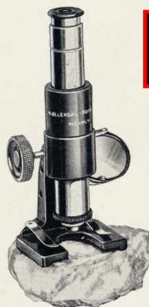
Above: Either microscope instantly detachable from base for examining surface of bulky objects.
